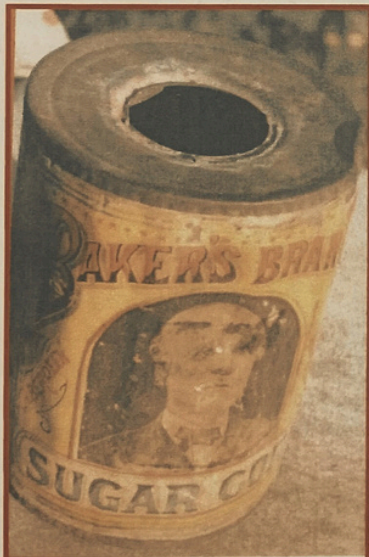
G.W. Baker soldered tin can, circa 1875. In the early days of canning, tin cans were filled through a small hole in the top. Then a cap was soldered onto it with lead solder. Later, the entire lid was crimped tightly in place, removing the need for solder and making for a healthier product.
